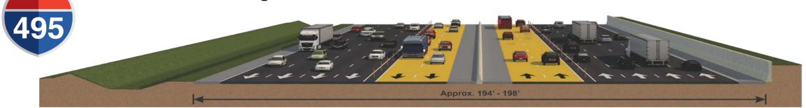
Convert existing HOV lane to HOT managed lane and add one HOT managed lane in each direction on I-270 between I-495 and I-370 and the I-270 East Spur from MD 187 to I-270
