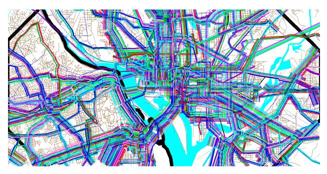
Figure 46 Using the pk\_vol.dbf file in Cube Base as the transit layer: All transit routes turned on, but non-transit links (modes 11-16) turned off
