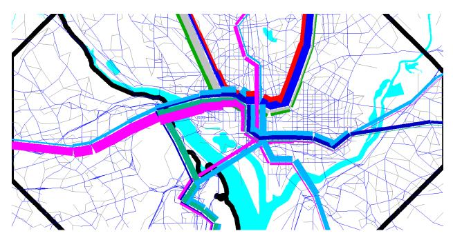
Figure 48 Using the pk\_vol.dbf file in Cube Base as the transit layer: Only mode-3 (Metrorail) links turned on; using multibandwidth to represent transit loads (ab\_vol): Arlington and DC
