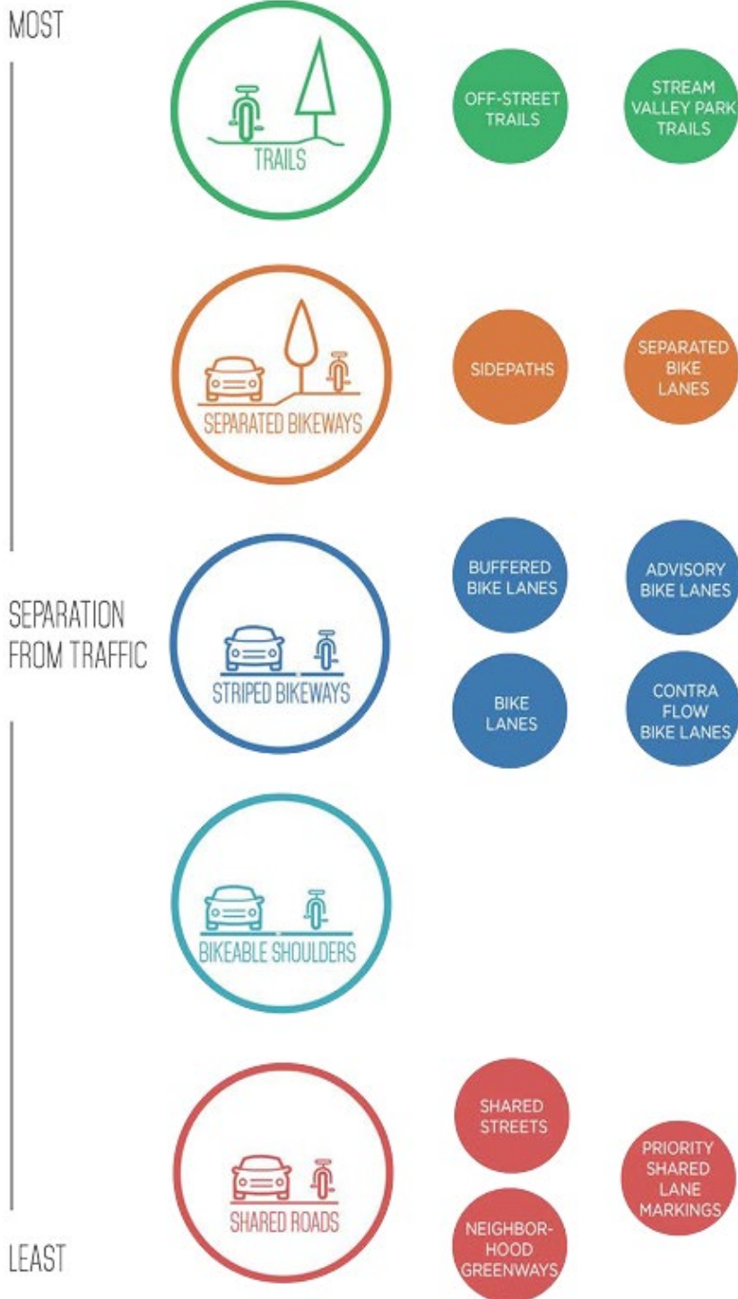
Figure 30 Bicycle Facility Classification
