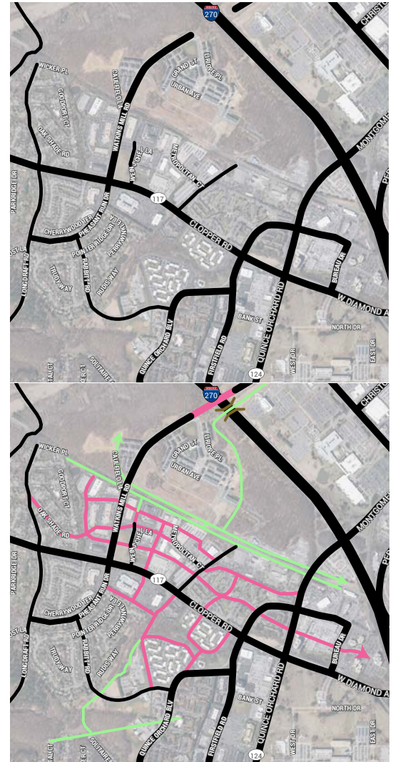
Top: Existing general street grid Bottom: Potential new street connections shown in pink. New trails shown in green.
