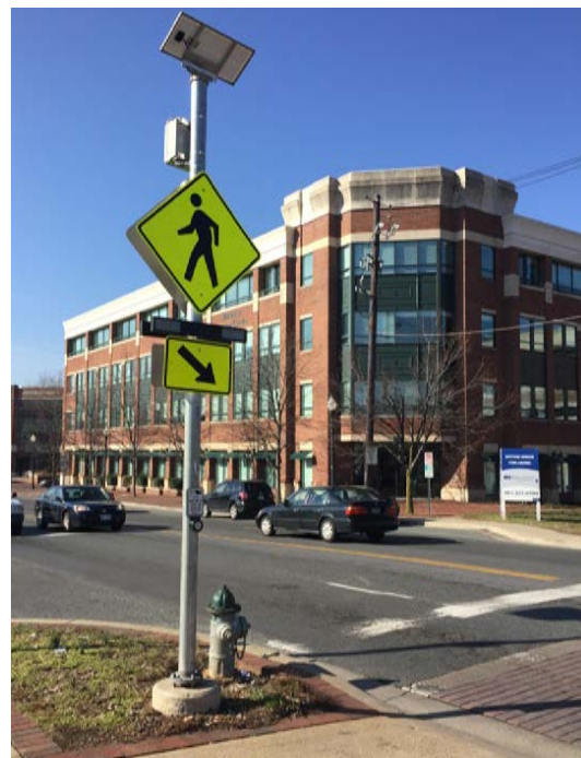
A Rectangular Flashing Beacon at Wells Avenue and South Summit Avenue confuses pedestrians and motorists when paired with a traffic signal
