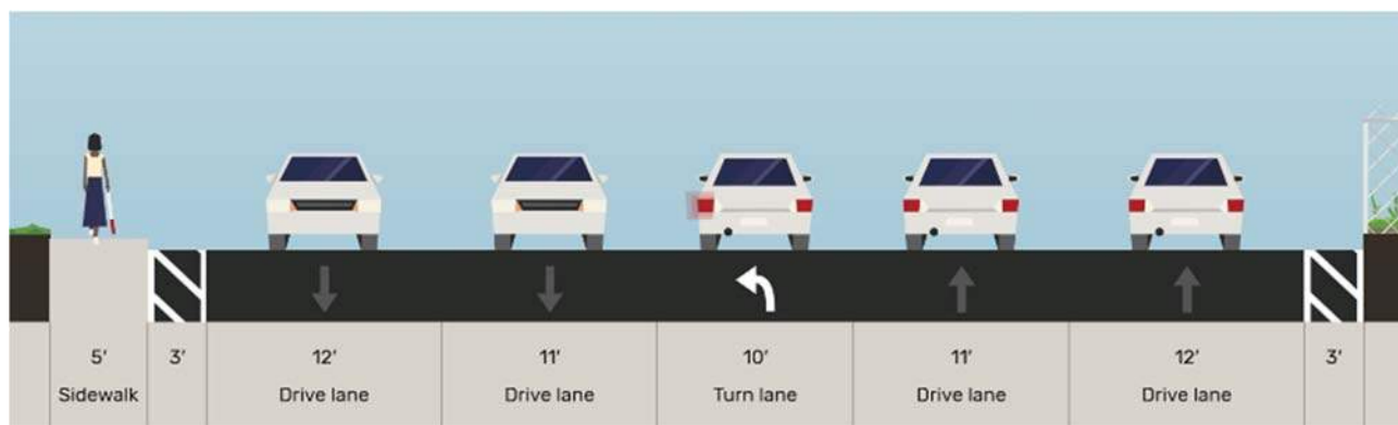
Figure 6. Intersection Typical Section
