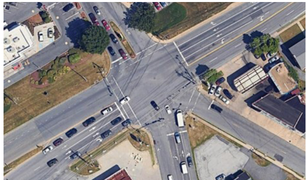
Figure 1-7: Jefferson St at Prospect Blvd/Pearl St is a five-legged intersection with more conflict points & complex phasing
