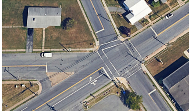
Figure 1-5: Jefferson St at Braddock Ave/Catoctin Ave is a five-legged intersection with more conflict points & complex phasing
