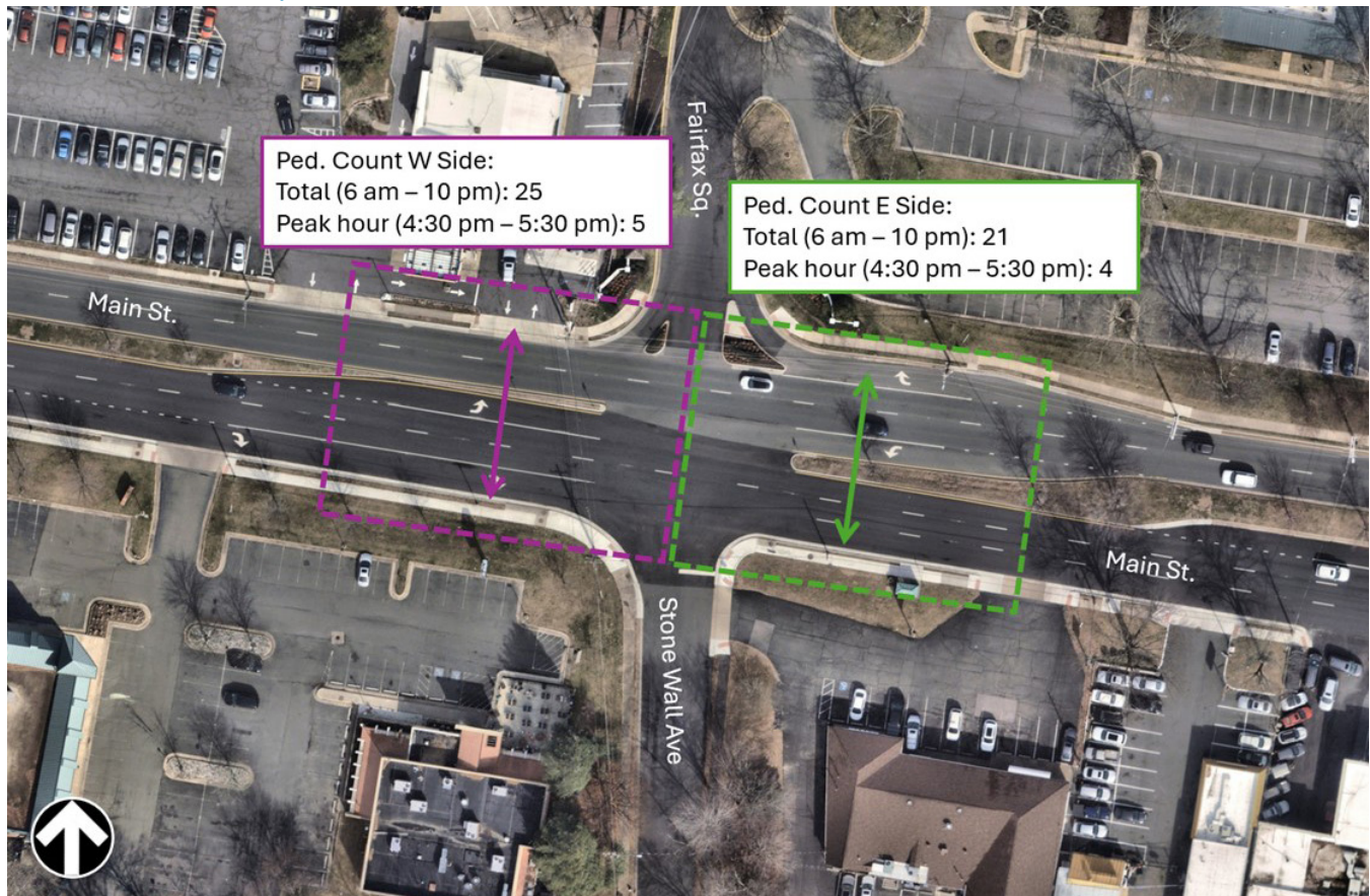
Figure 5. Pedestrian count data collected at the intersection of Main Street and Stone Wall Avenue / Fairfax Square
