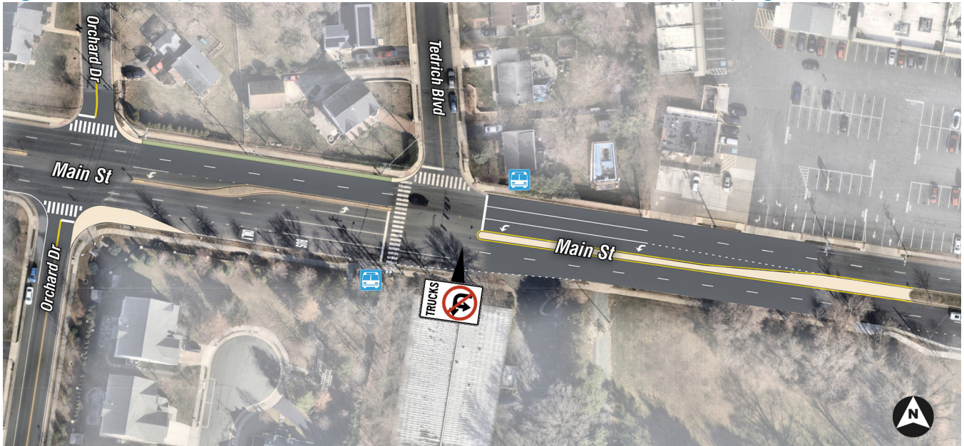
Figure 58. Concept for median closure in front of the Main Street Shopping Center
