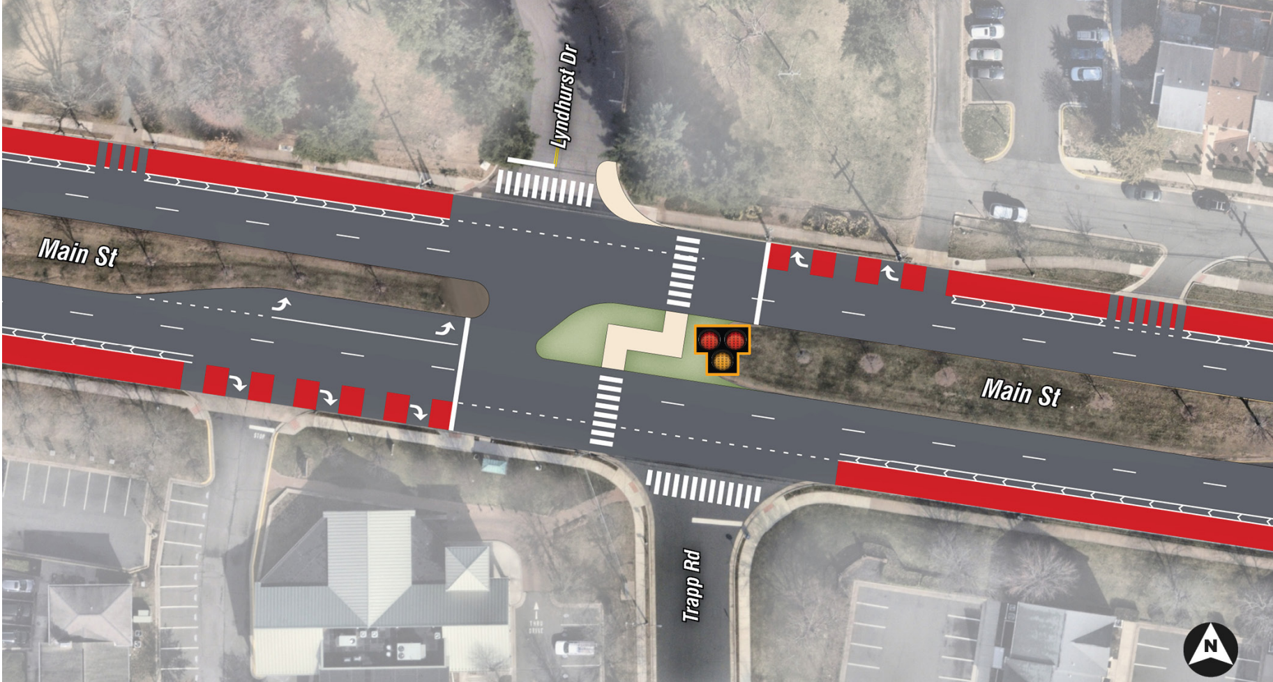
Figure 54. Potential concept for extended median on Main Street at Trapp Road / Lyndhurst Drive, relocated crosswalk, and new PHB
