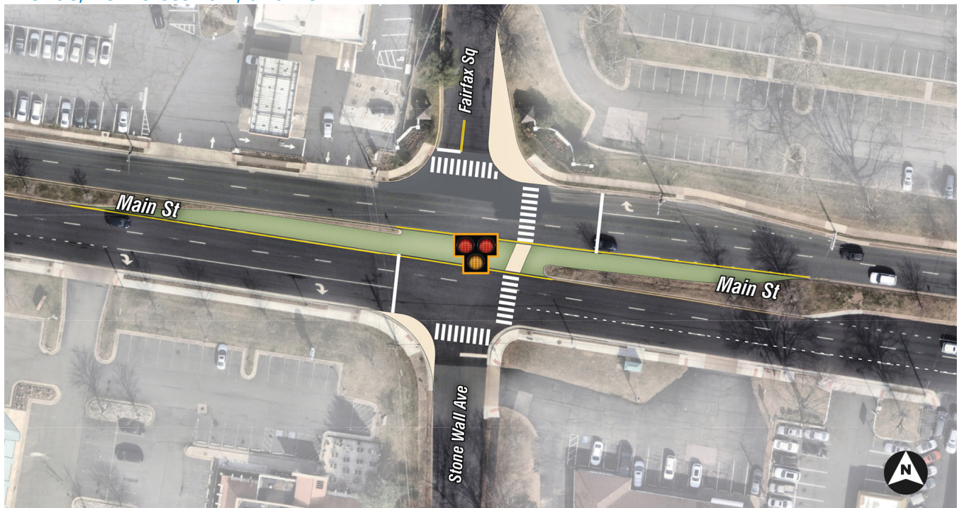
Figure 56. Potential concept for median closure on Main Street at Fairfax Square / Stone Wall Avenue, new crosswalk, and new PHB
