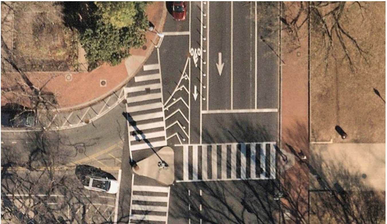
Figure 48. Example of curb extension with temporary materials at 11th Street and East Capitol Street in Washington, DC (Source: Nearmap)
