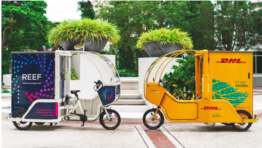
Figure 4: E-Cargo Bike with Mini Shipping Trailer and Weather Protection
