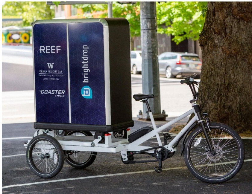
Figure 3: E-Cargo Bike with a Mini Shipping Trailer
