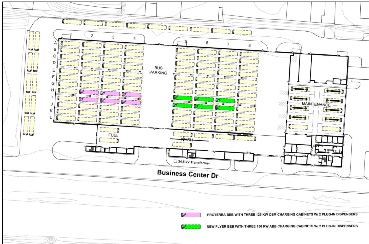
Exhibit 8: Initial BEB Charging Configuration
