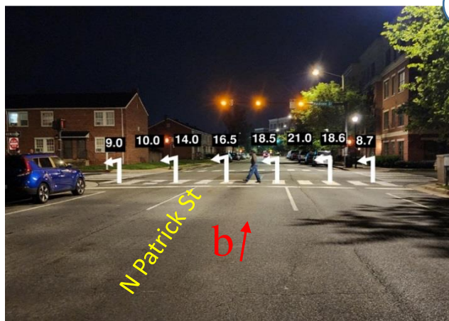
Figure 8. Vertical Illuminance Readings (lux) in Crosswalks at Patrick and Madison Streets (A: Aerial view; B: Street / Approach View) - (Red arrow shows direction of travel and white arrows show light-meter orientation).
