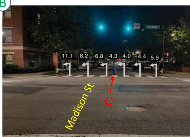
Figure 8. Vertical Illuminance Readings (lux) in Crosswalks at Patrick and Madison Streets (A: Aerial view; B: Street / Approach View) - (Red arrow shows direction of travel and white arrows show light-meter orientation).
